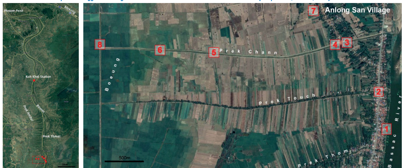
Figure 7. COSTEA Monitoring site on the right bank of the Bassac Point 1 to 6 and 8 are pressure loggers allowing to measure water levels. Point 7 is a weather station (Temperature, rainfall, wind)
