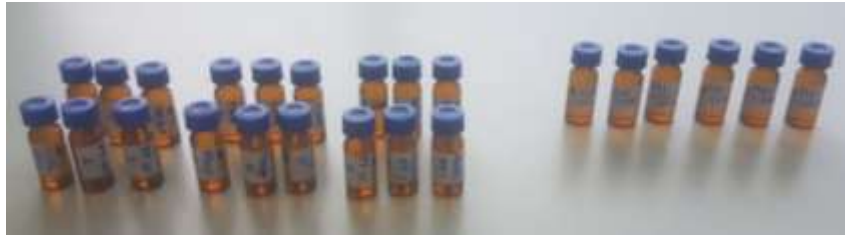
Figure B3. The 18 water samples and the 6 standards solution, ready for analysis
